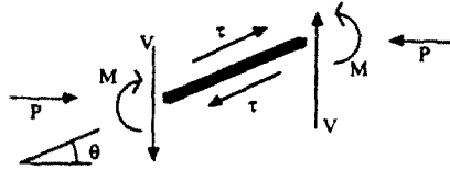
Fig. 2. Free-body diagram of an element of a micro-buckling fiber.
